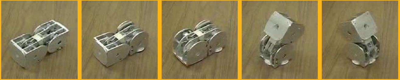
An iRobot module has four degrees of freedom. It can stand on its own, for instance, and if it was equipped with a camera, could scan its environment.
