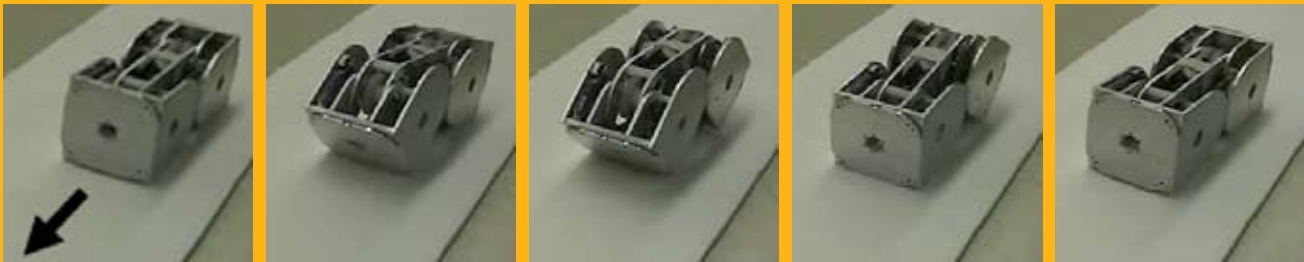
One of iMobot's modes of locomotion is an inch-worming crawl demonstrated in this photo sequence.
