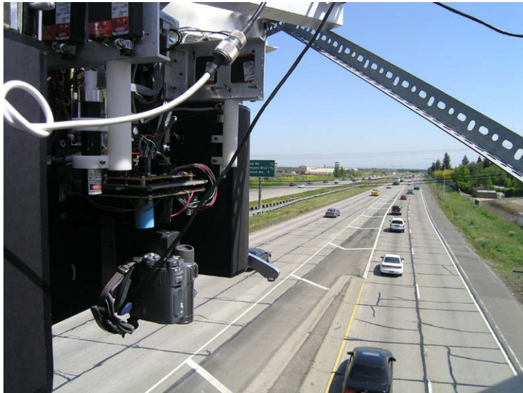
Fig. 6. A laser-based highway detection system.
