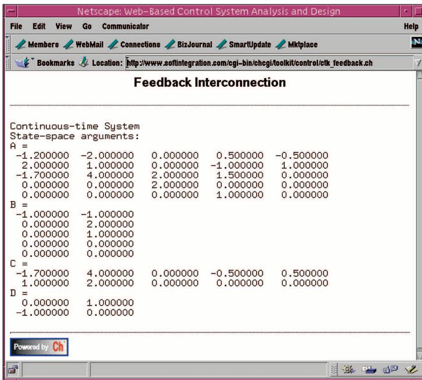
**Figure 12.** The state space matrices of the feedback system shown in Figure 11. The feedback system is a MIMO system with two inputs and two outputs. The system has five state variables.
