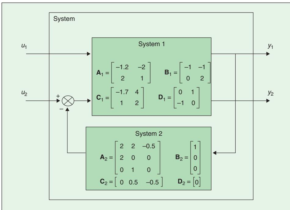
**Figure 11.** A feedback system involving two subsystems. The plant subsystem is a MIMO system. The feedback controller is a SISO system.
