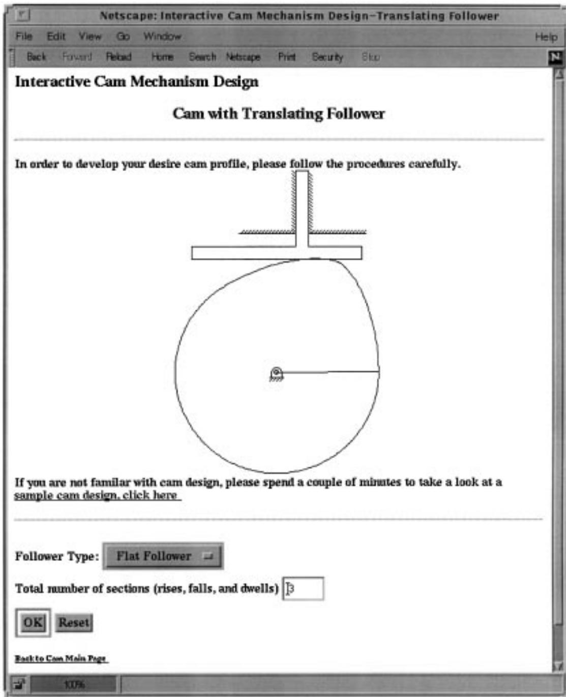
Fig. 2. Selection of the number of cam sections.
