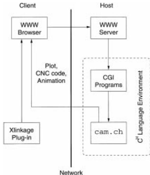
Fig. 13. System architecture for CGI-based cam design.
