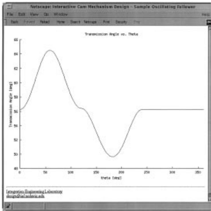
Fig. 28. Oscillating follower transmission angle.
