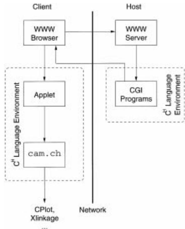
Fig. 12. System architecture for applet-based cam design.
