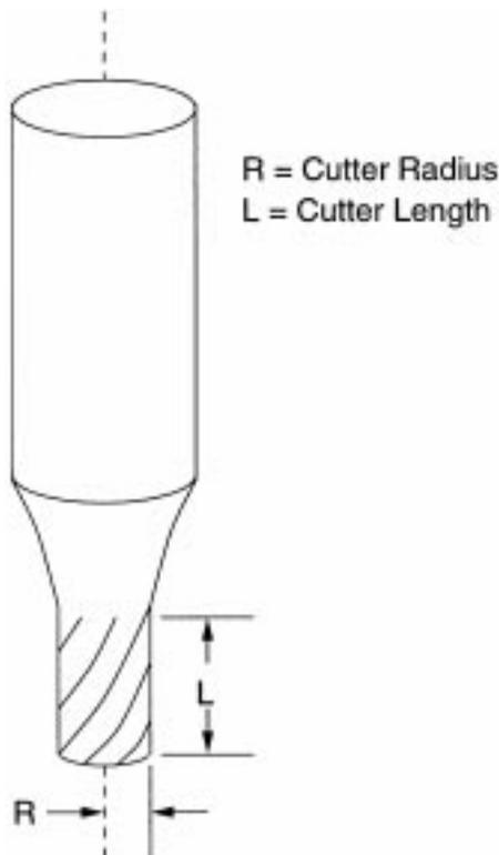
Fig. 10. Cutter dimensions.
