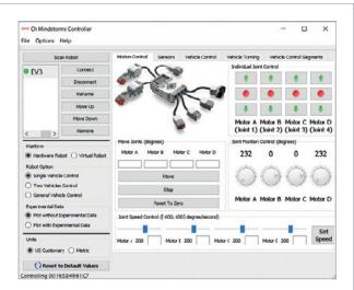
Above The Motion Control panel features many options for individual motor control, and displays information about the current positions of each motor
