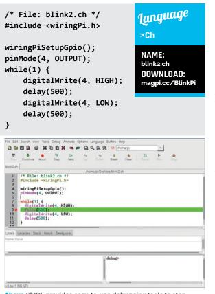
Above ChIDE provides easy-to-use debugging tools to step through Ch code
